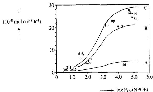
Figure 7. Effect of carrier lipophilicity on the flux for different values of  $K_m$ : (A)  $K_m = 10^3 \text{ M}^{-1}$ ; (B)  $K_m = 10^4 \text{ M}^{-1}$ ; (C)  $K_m = 5 \times 10^4 \text{ M}^{-1}$ .
