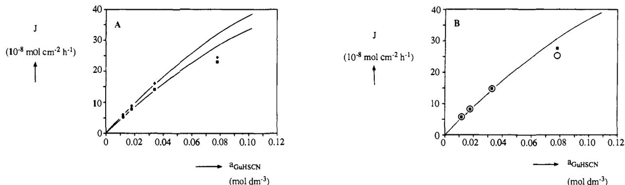
**Figure 9.** Theoretical curves of the flux vs the initial salt concentration (aqueous phase) and the experimental fluxes for the carriers: (A) **9**,  $K_m = 9.6 \times 10^4 \text{ M}^{-1}$  (■), **11**,  $K_m = 9.6 \times 10^4 \text{ M}^{-1}$  (◆); (B) **12**,  $K_m = 8.9 \times 10^4 \text{ M}^{-1}$  (■), **14**,  $K_m = 8.7 \times 10^4 \text{ M}^{-1}$  (○).
