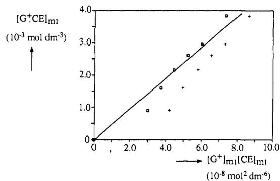
**Figure 5.**  $[G^+CE]_{m1}$  as function of  $[G^+]_{m1}[CE]_{m1}$  for crown ether **11** by variation of the initial crown ether concentration, according to model A (+) and B (□).
