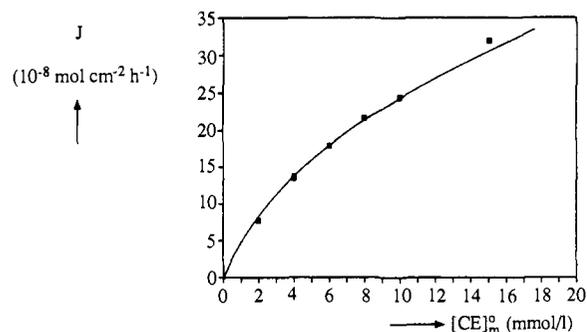
Figure 6. Theoretical curve of the flux vs the initial crown ether concentration, according to model B, and the experimental (■) values for carrier 11.
